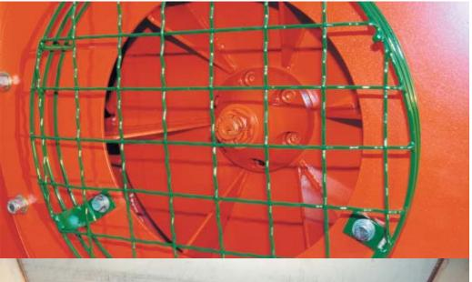
24" diameter centrifugal fan, dynamically balanced. Fan is driven directly by a (2) speed gearbox with heavy duty fan shaft bearings.
