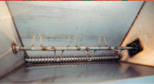
300 lb. capacity hopper of heavy gauge stainless steel construction with a hinged/ locking stainless steel cover. The agitator assembly and auger assembly are also made of stainless steel. The agitator and auger are driven directly by hydraulic motors: no chain or belt drive. The agitator can be run with or without the auger. The speed controls for agitator and auger are separate.
